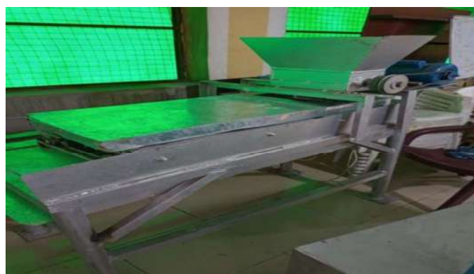
Plate 5. Fabricated Motorised Dewatered Cassava Mash Sifting Machine
