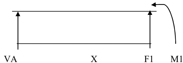
Fig. 7. Forces on defibering shaft at section 1-1
